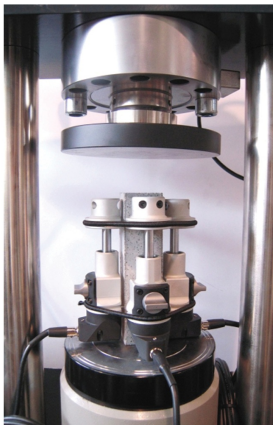
Three compressometer-extensometers 55-C0222/H fitted to a mortar prism 40x40x160 mm
